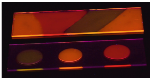
Fig. 6 (color online). Luminescent layer composed of different nanocomposite blends obtained by “painting” on glass and casting 150 \mu L drops of QD/polymer solutions on soda-lime glass ( d = 10 - 15 mm).
