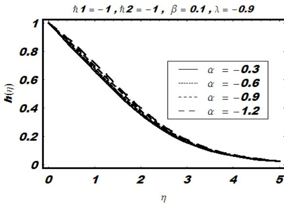
Fig. 8. Influence of shrinking parameter  $\alpha$  on  $h$  for two-dimensional stagnation flow.
