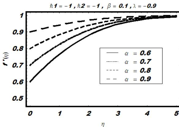
Fig. 5. Influence of stretching parameter  $\alpha$  on  $f$  for two-dimensional stagnation flow.
