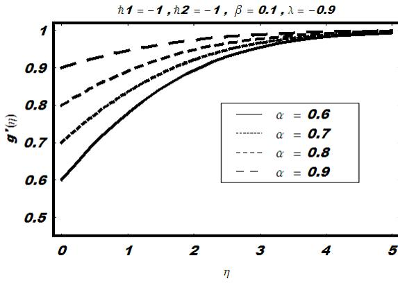
Fig. 13. Influence of stretching parameter  $\alpha$  on  $g$  for axisymmetric stagnation flow towards axisymmetric shrinking surface.
