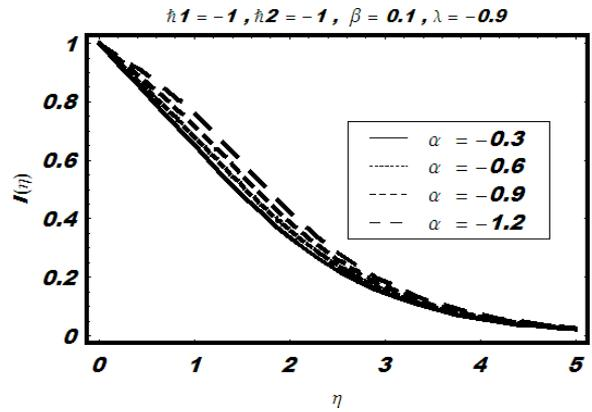
Fig. 16. Influence of shrinking parameter  $\alpha$  on  $l$  for axisymmetric stagnation flow towards axisymmetric shrinking surface.
