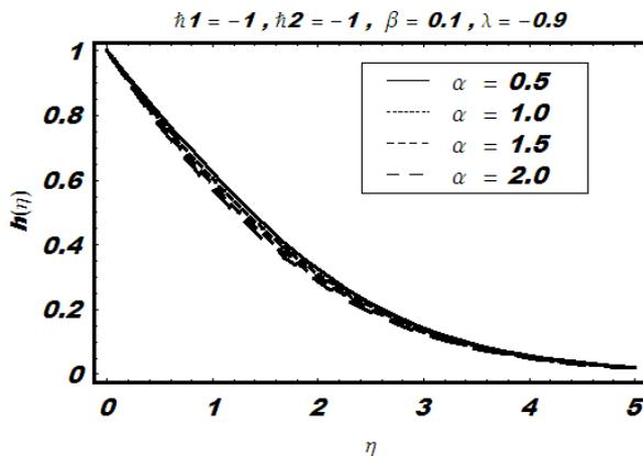
Fig. 6. Influence of stretching parameter  $\alpha$  on  $h$  for two-dimensional stagnation flow.
