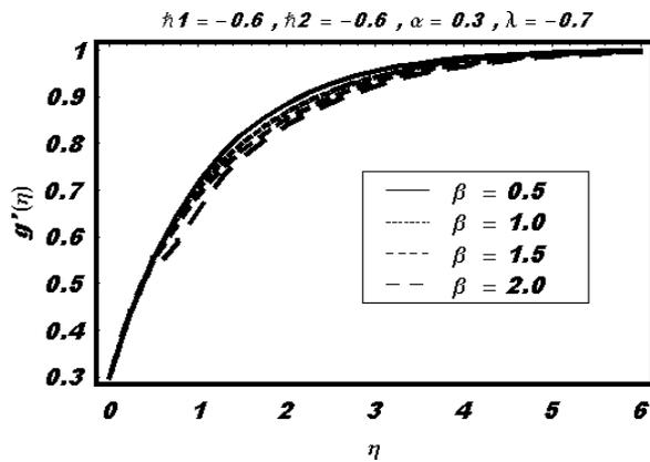
Fig. 19. Influence of  $\beta$  on  $g$  for axisymmetric stagnation flow towards axisymmetric shrinking surface.
