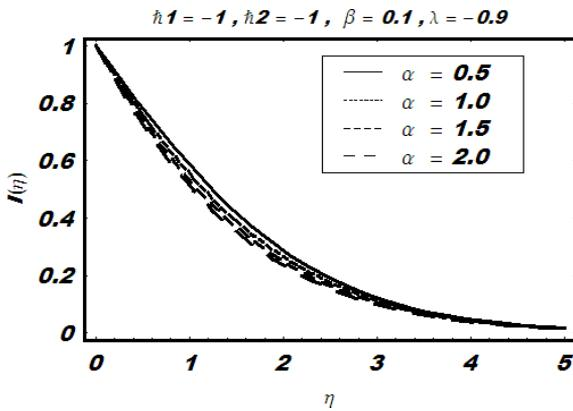
Fig. 14. Influence of stretching parameter  $\alpha$  on  $h$  for axisymmetric stagnation flow towards axisymmetric shrinking surface.
