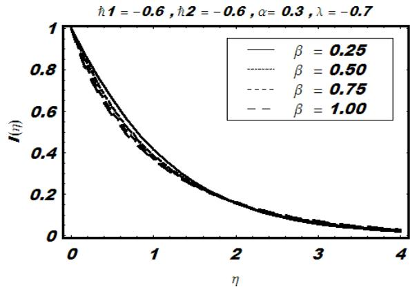
Fig. 20. Influence of  $\beta$  on  $l$  for axisymmetric stagnation flow towards axisymmetric shrinking surface.
