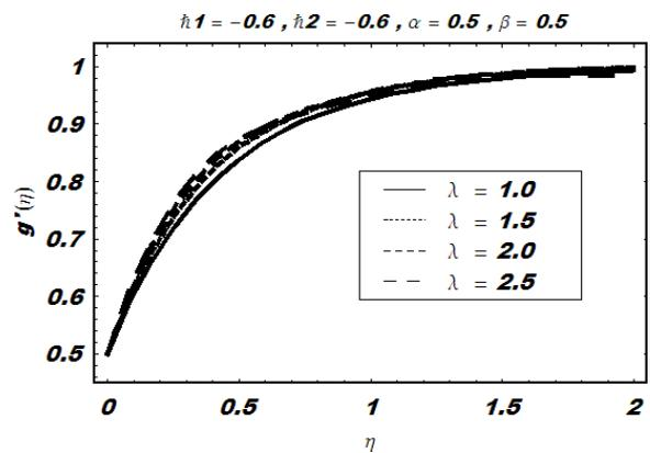
Fig. 17. Influence of  $\lambda$  on  $g$  for axisymmetric stagnation flow towards axisymmetric shrinking surface.
