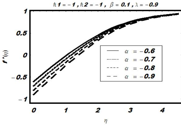
Fig. 7. Influence of shrinking parameter  $\alpha$  on  $f$  for two-dimensional stagnation flow.
