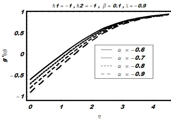
Fig. 15. Influence of shrinking parameter  $\alpha$  on  $g$  for axisymmetric stagnation flow towards axisymmetric shrinking surface.
