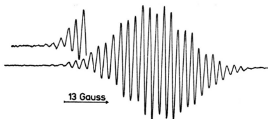
Figure. First-derivative ESR spectrum of 5 , Ar = p -C 6 H 5 NO 2 , X = NMe 2 , in methylene dichloride at -40 °C.
